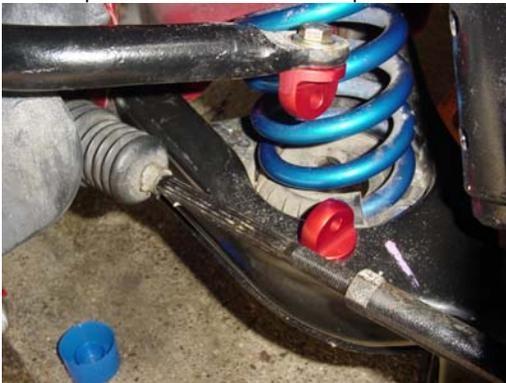
4. Install Powergrid Adjustable Links with proper relationship to the mounts.
