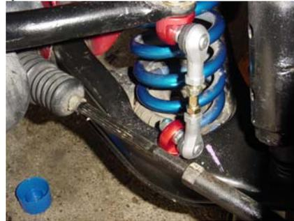
6. Check steering travel lock to lock to insure clearance of the link system. Reposition if necessary.
